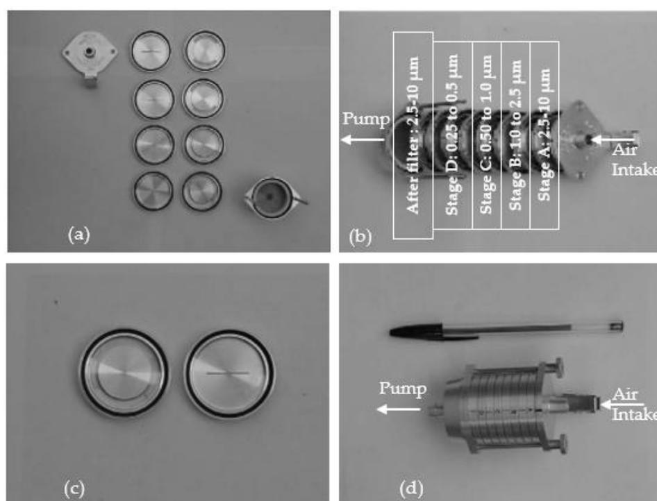
**Figure 15.** Visual representation of a Personal Cascade Impactor Sampler (PCIS); (a) Dismantled view of interior sections of PCIS (b) Schematic representation of the five interior sections of a PCIS, (c) Zoomed dismantled view of interior section, (d) Picture of PCIS unit, pen placed for perspective of size [303].
