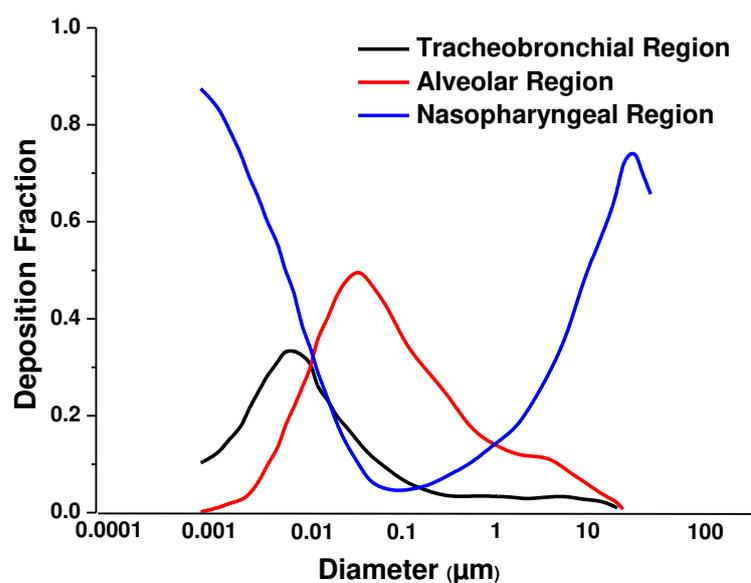
Figure 3. Deposition of particles according to size distribution.
