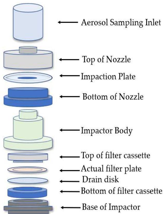
**Figure 11.** PM<sub>2.5</sub> Harvard Impactor collector.
