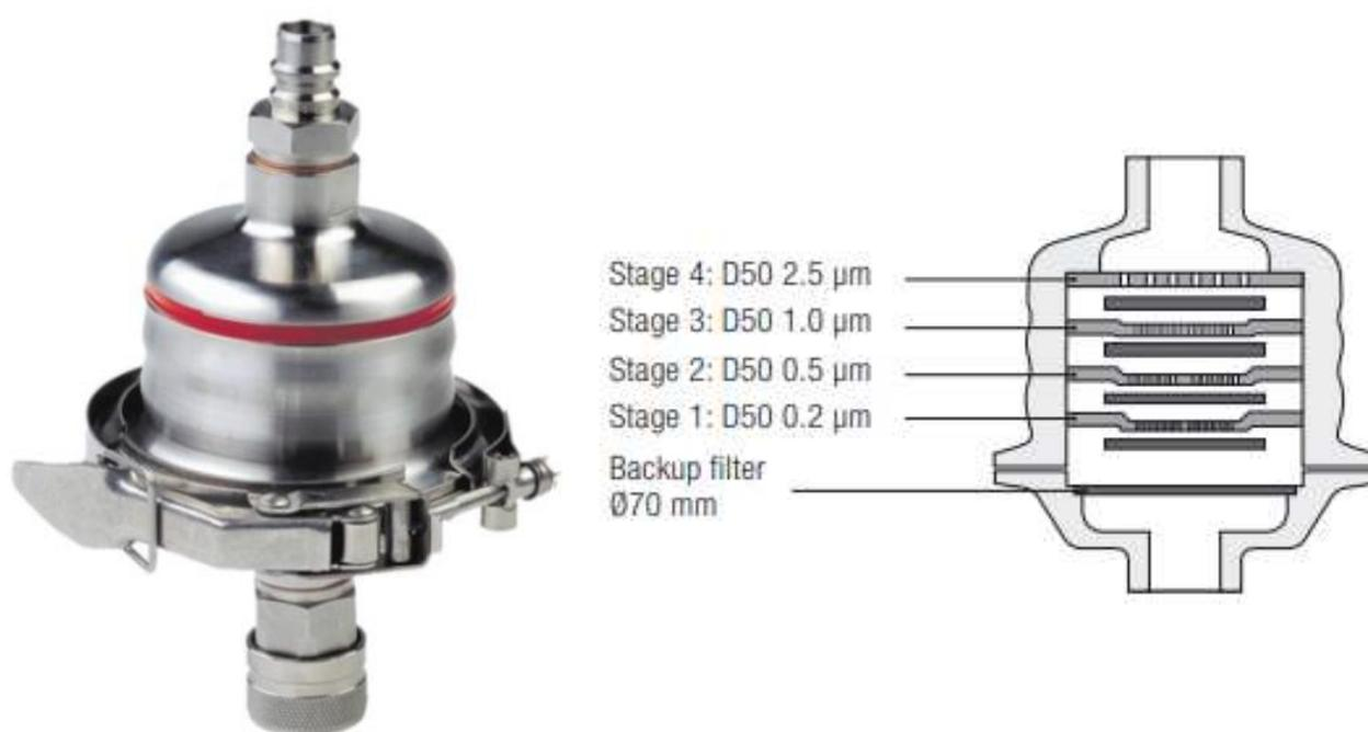
**Figure 13.** Visual representation of DGI (Dekati gravimetric impactor, 70 LPM) [285].
