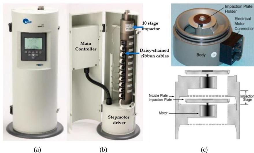
**Figure 14.** Visual representation of a MOUDI II Impactor Model. (a) View of Model 120R MOUDI II Impactor. (b) View of Model 120R MOUDI II Impactor parts of the instrument. (c) Motor with impactor stage, and its internal view [293].
