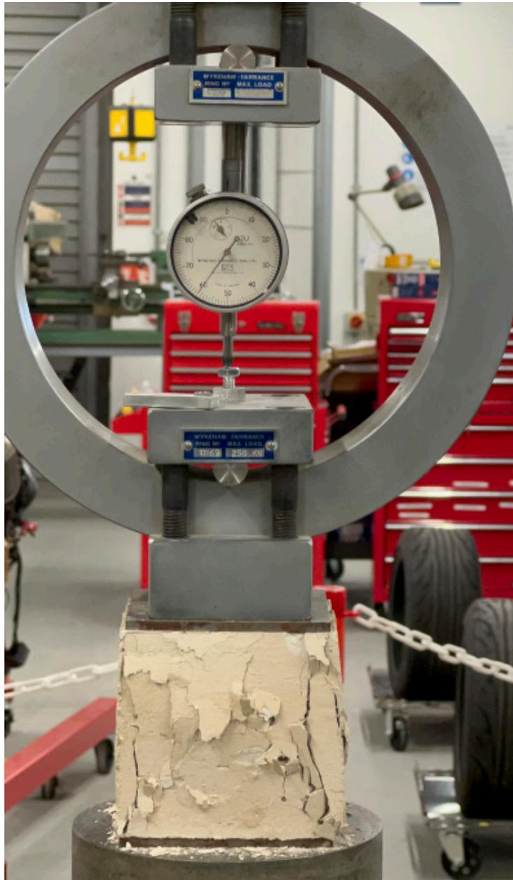
Fig.44 - Lime Block Being Tested for Compressive Strength
