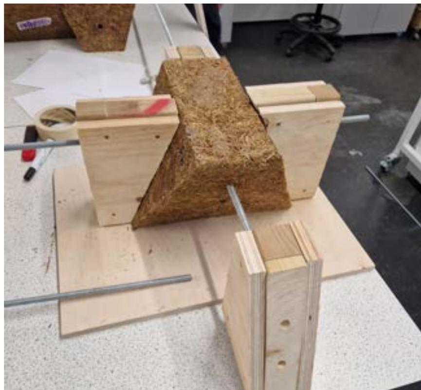
Whilst the geometric pattern is designed to be interlocking and self-supporting, there is still a limit to the stability of the structure without the addition of tension rods.
