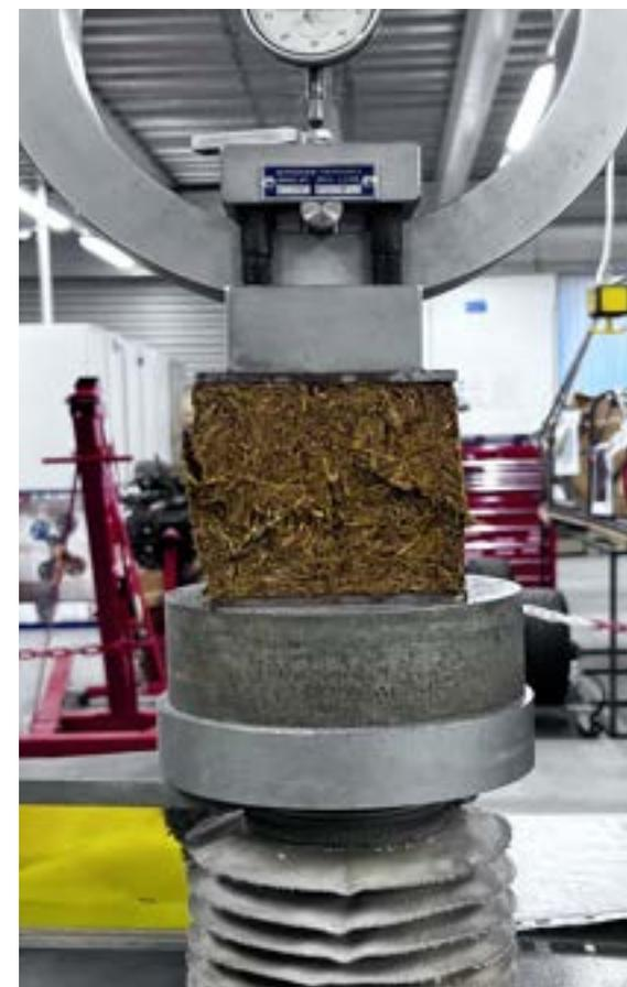
Fig.34 - Compression Test Machine With Proving Ring
