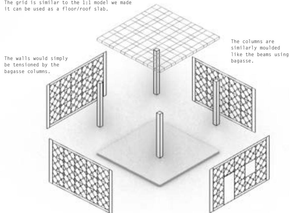
The walls would simply be tensioned by the bagasse columns.
