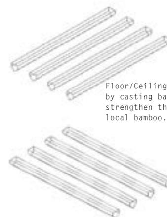
Floor/Ceiling beams can be constructed by casting bagasse in moulds. To further strengthen the beam, they can be thread with local bamboo.
