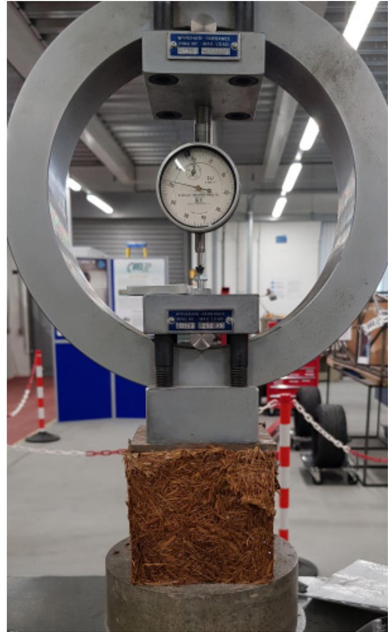
Fig.45 - Bagasse and Sodium Silicate Block Being Tested for Compressive Strength
