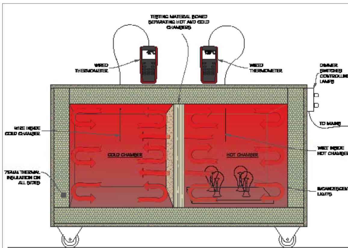
Fig.47 - Thermal Testing Rack Diagram
