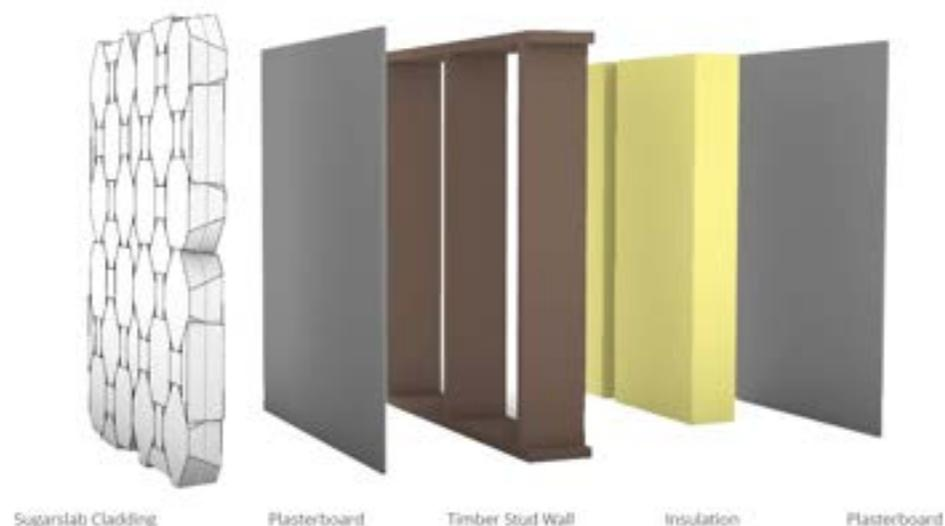
Fig.81 - Axonometric Exploded Construction Section
