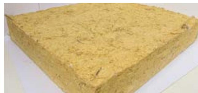
Fig.49 - Sugarslab Board 75mm
