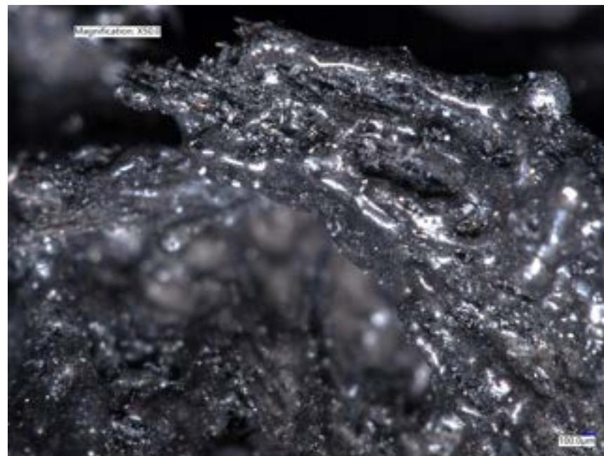
Fig.28 - Microscoping Image at X50.00 of Sugarslab after Fire Test
