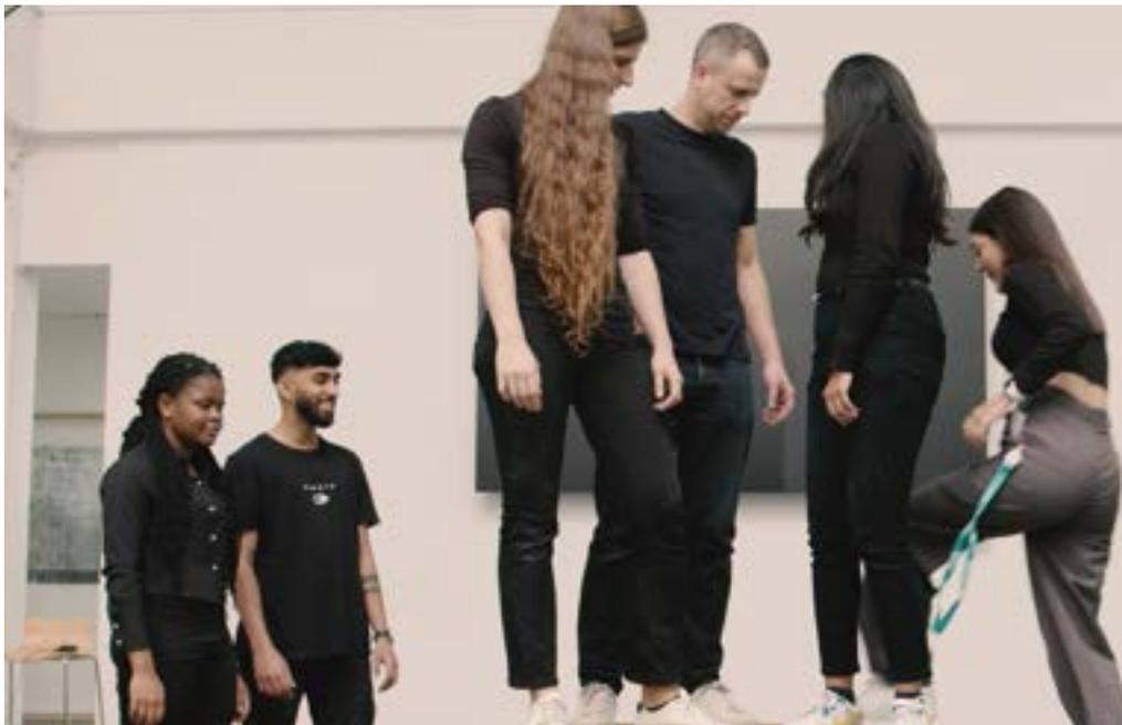
To test the structural stability of the slab with the tension support rods we gradually loaded with weight in the form of people.
