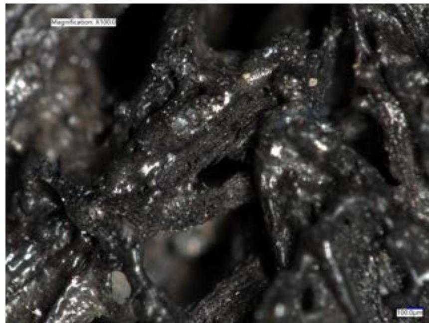
Fig.27 - Microscoping Image at X100.00 of Sugarslab after Fire Test
