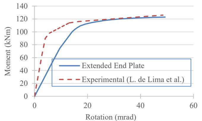
Figure 10. IPE to HEB extended end plate joint FE model comparison with experimental results
