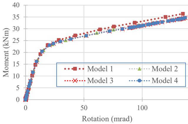
Figure 7. Mesh sensitivity analysis: moment-rotation response.
