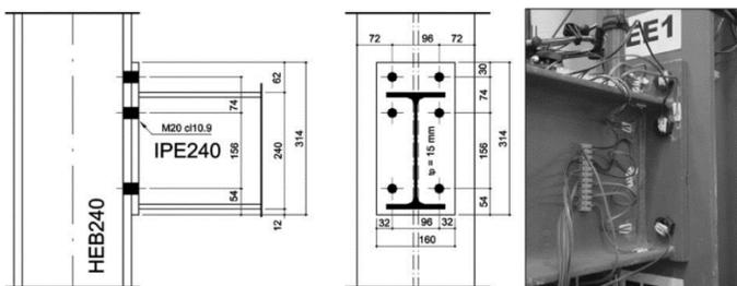
Figure 2. Joint detailing for extended end plate beam-to-column joint by de Lima *et al.* (de Lima et al. 2004)
