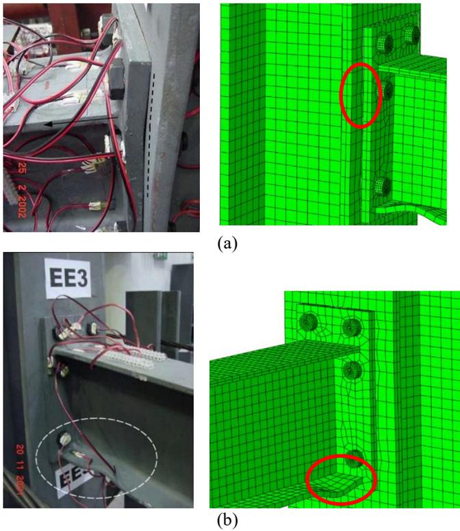
Figure 11. Comparison of failure modes for extended end plate joint with experiments in (de Lima et al. 2004): (a) End plate bending; (b) Beam bottom flange bending
