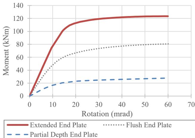
Figure 12. Moment-rotation behaviour of IPE to HEB end plate bolted joints (joint rotation limited to 60 mrad for comparison)
