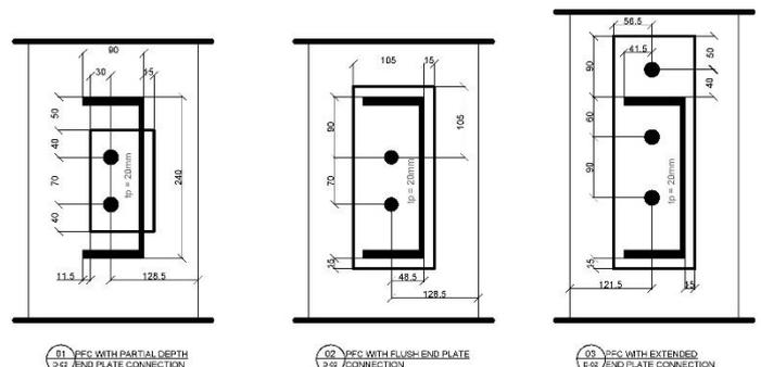
Figure 4. UPE 240 (PFC) Beam to SHS 250×250×16 Column bolted end plate connection details
