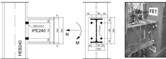
Figure 1. Connection detail for flush end plate bolted joint used by da Silva *et al.* (Simões Da Silva et al. 2004)
