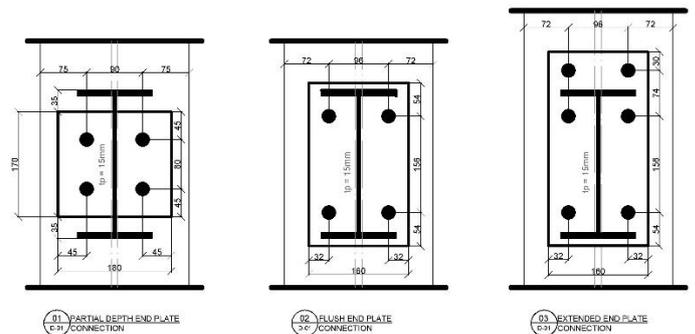
Figure 3. IPE 240 Beam to HEB 240 Column end plate bolted connection details
