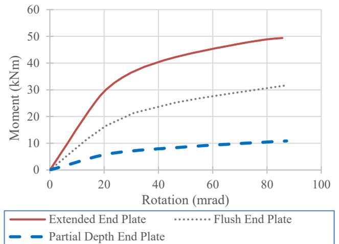
Figure 13. Moment-rotation behaviour of PFC-SHS end plate bolted joints (Joint rotation limited to 85 mrad for comparison)
