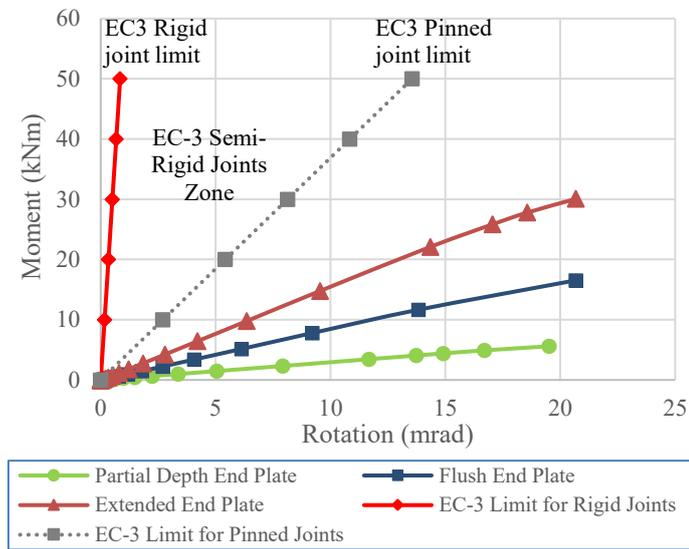
Figure 15. Joint classification as per EC 3 for PFC-SHS joints
