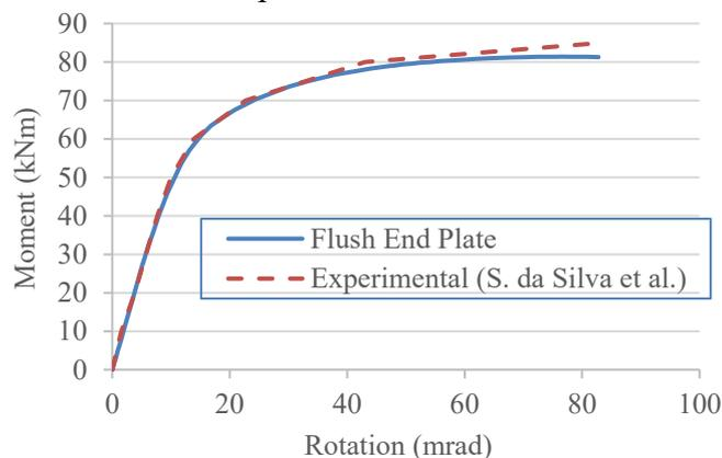
Figure 8. IPE to HEB flush end plate joint FE model comparison with experimental results
