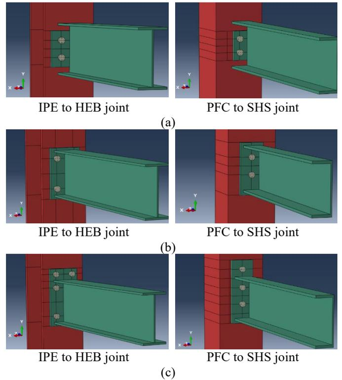
Figure 6. Assembled ABAQUS beam-to-column models (a) Partial depth end plate (b) Flush end plate (c) Extended end plate
