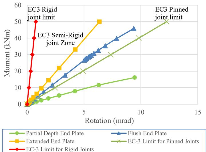
Figure 14. Joint classification as per EC 3 for IPE-HEB joints
