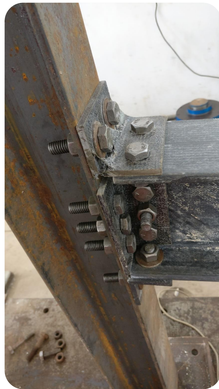
5. SFFc2: Bolted joint with FRP web and flange cleats
