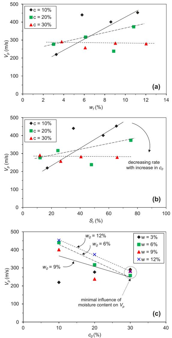
Figure 3. Variation of  $V_p$  with: (a)  $w_f$ ; (b)  $S_r$  and (c)  $c_0$ .
