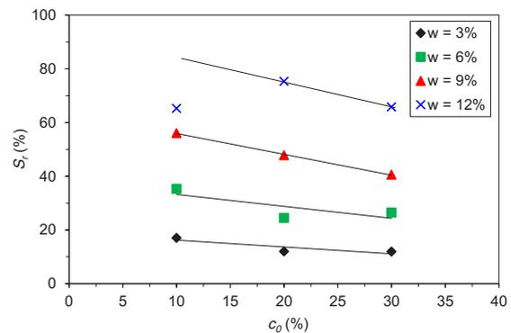
Figure 5. Variation of degree of saturation with clay content
