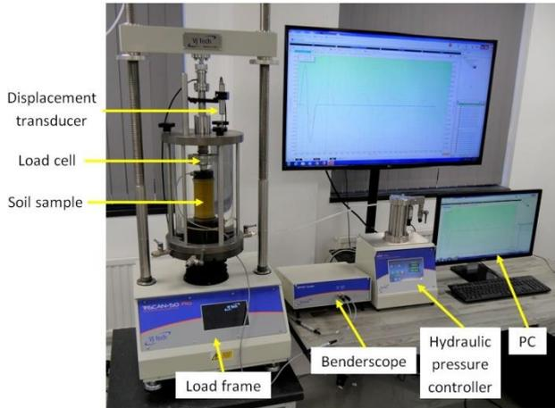
Figure 1. Bender element setup for triaxial testing equipment
