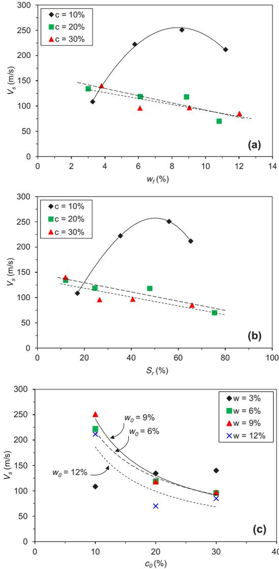
Figure 2. Variation of  $V_s$  with: (a)  $w_f$ ; (b)  $S_r$  and (c)  $c_0$ .
