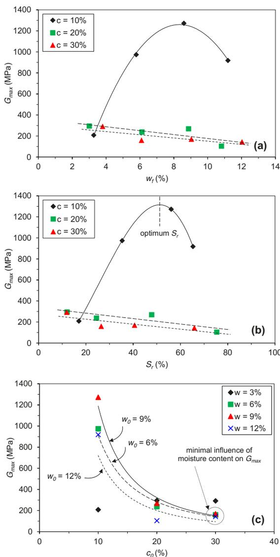
Figure 4. Variation of  $G_{max}$  with: (a)  $w_f$ ; (b)  $S_r$  and (c)  $c_0$ .
