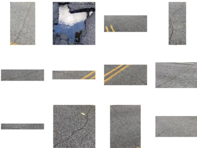
Fig. 3. Collage of Images in the Transverse Crack Category
