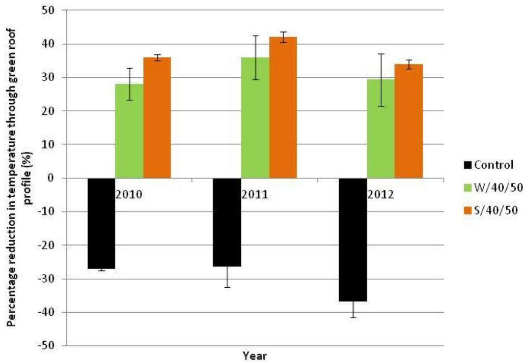
**Figure 26.** Average percentage reduction in temperature through control, W/40/50 and S/40/50 green roof profiles for the month of July, 2010 to 2012. Reduction in temperature calculated from the difference in temperature between sensor 4 (above the roof) and sensor 1 (beneath the roof). Error bars represent the standard error of the mean ( $n = 3$ ).
