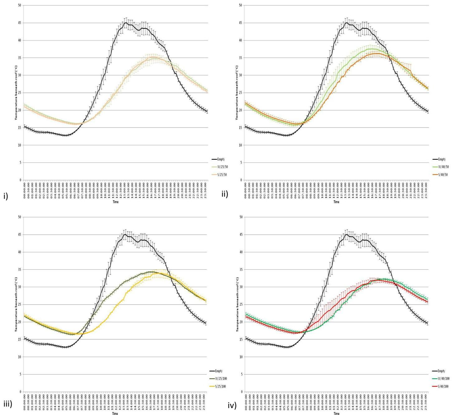
**Figure 24. Average temperature immediately above the green and control roofs at Barking Riverside on one of the hottest day of 2013 (13th July) [Data for hottest day unavailable due to power cut on site].** i) Green roof pair W/25/50 and S/25/50; ii) Green roof pair W/40/50 and S/40/50; iii) Green roof pair W/25/100 and S/25/100; iv) Green roof pair W/40/100 and S/40/100. Error bars represent the standard error of the mean ( $n = 3$ ).
