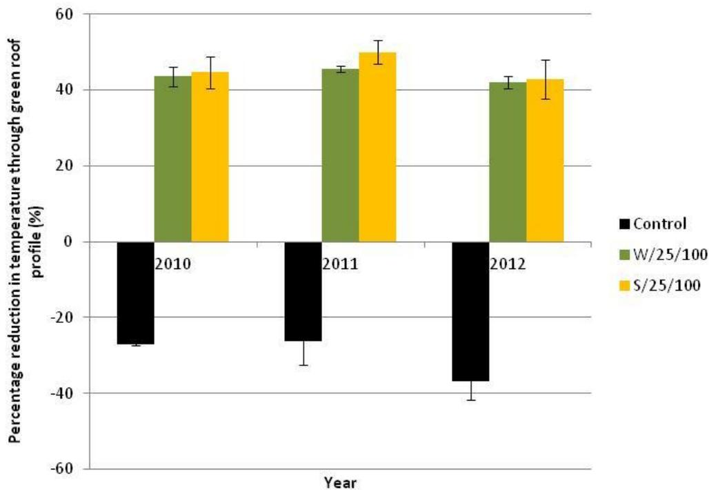
**Figure 27.** Average percentage reduction in temperature through control, W/25/100 and S/25/100 green roof profiles for the month of July, 2010 to 2012. Reduction in temperature calculated from the difference in temperature between sensor 4 (above the roof) and sensor 1 (beneath the roof). Error bars represent the standard error of the mean ( $n = 3$ ).
