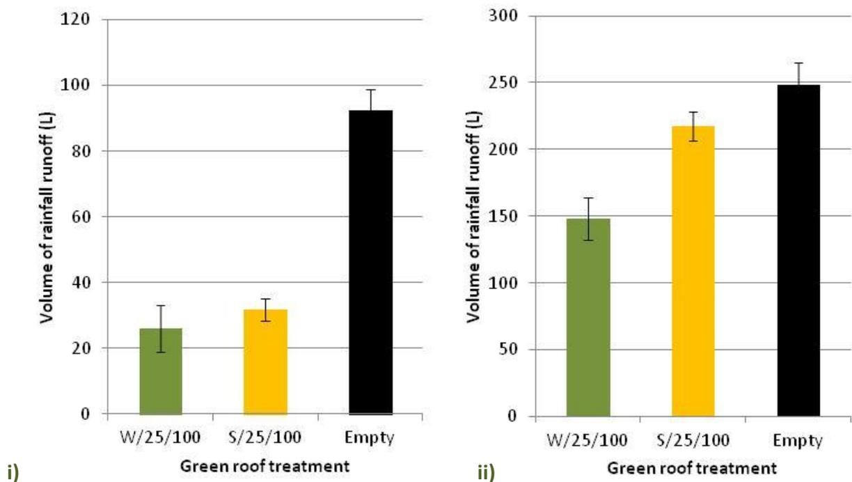
**Figure 15.** Average percentage rainfall attenuation for empty control roofs and 25 mm drainage, 100 mm substrate sedum and wildflower roofs at Barking Riverside for i) the summer months July to September 2010, and ii) the winter months October to December 2010. Error bars represent the standard error of the mean ( $n = 3$ ).
