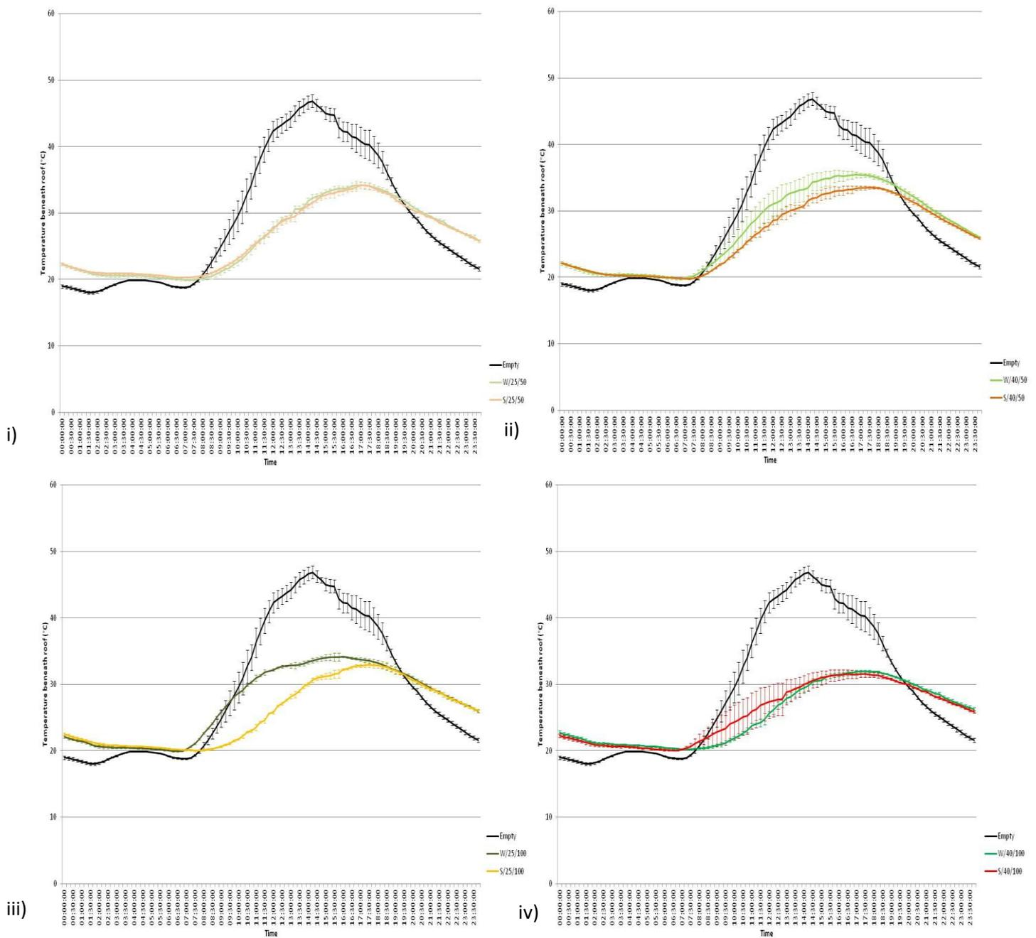
**Figure 23. Average temperature immediately beneath each green and control roofs at Barking Riverside on the hottest day of 2012 (18th August). i) Green roof pair W/25/50 and S/25/50; ii) Green roof pair W/40/50 and S/40/50; iii) Green roof pair W/25/100 and S/25/100; iv) Green roof pair W/40/100 and S/40/100. Error bars represent the standard error of the mean ( $n = 3$ ).**
