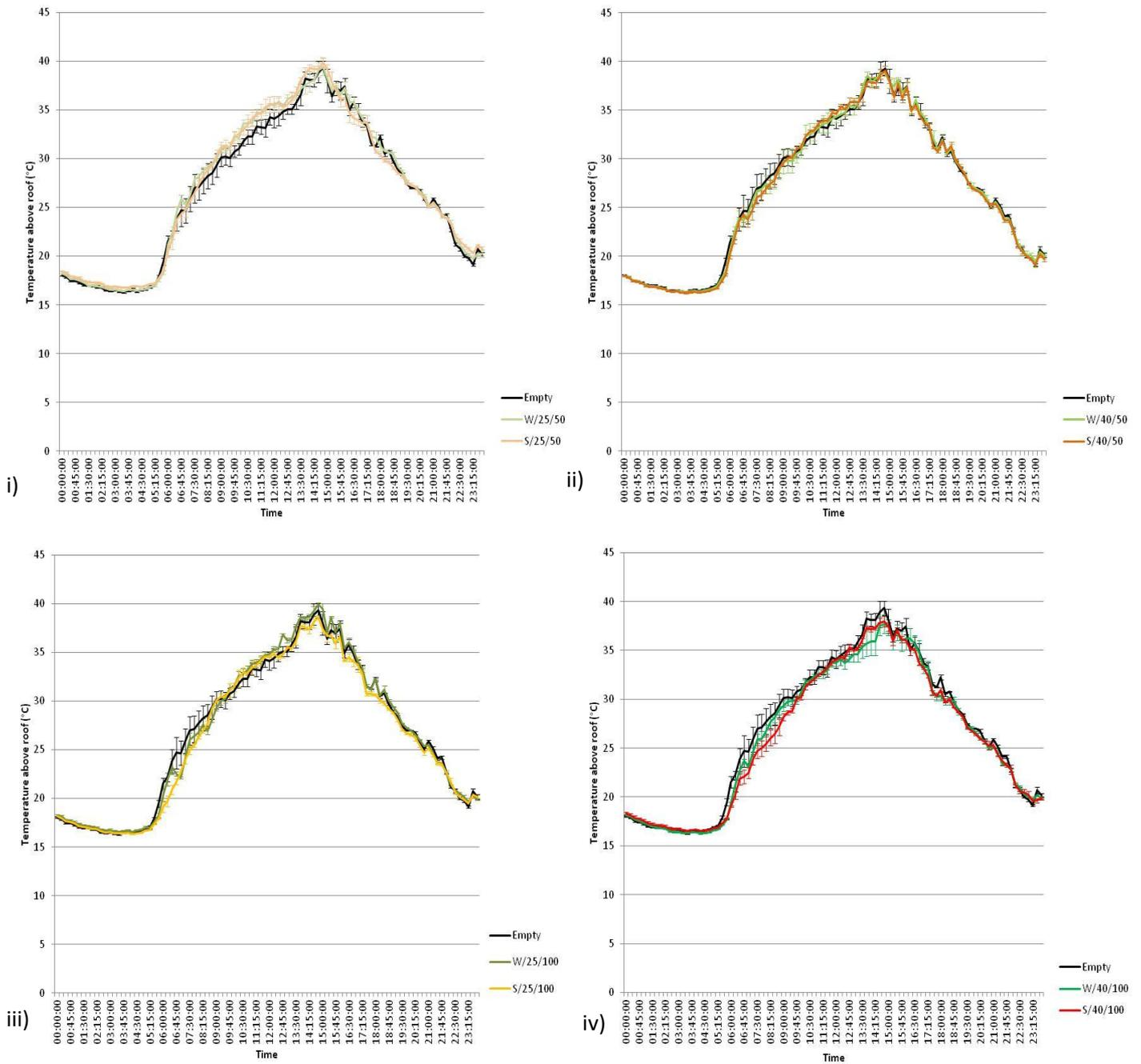
**Figure 18. Average temperature immediately above the green and control roofs at Barking Riverside on the hottest day of 2011 (27th June).** i) Green roof pair W/25/50 and S/25/50; ii) Green roof pair W/40/50 and S/40/50; iii) Green roof pair W/25/100 and S/25/100; iv) Green roof pair W/40/100 and S/40/100. Error bars represent the standard error of the mean ( $n = 3$ ).
