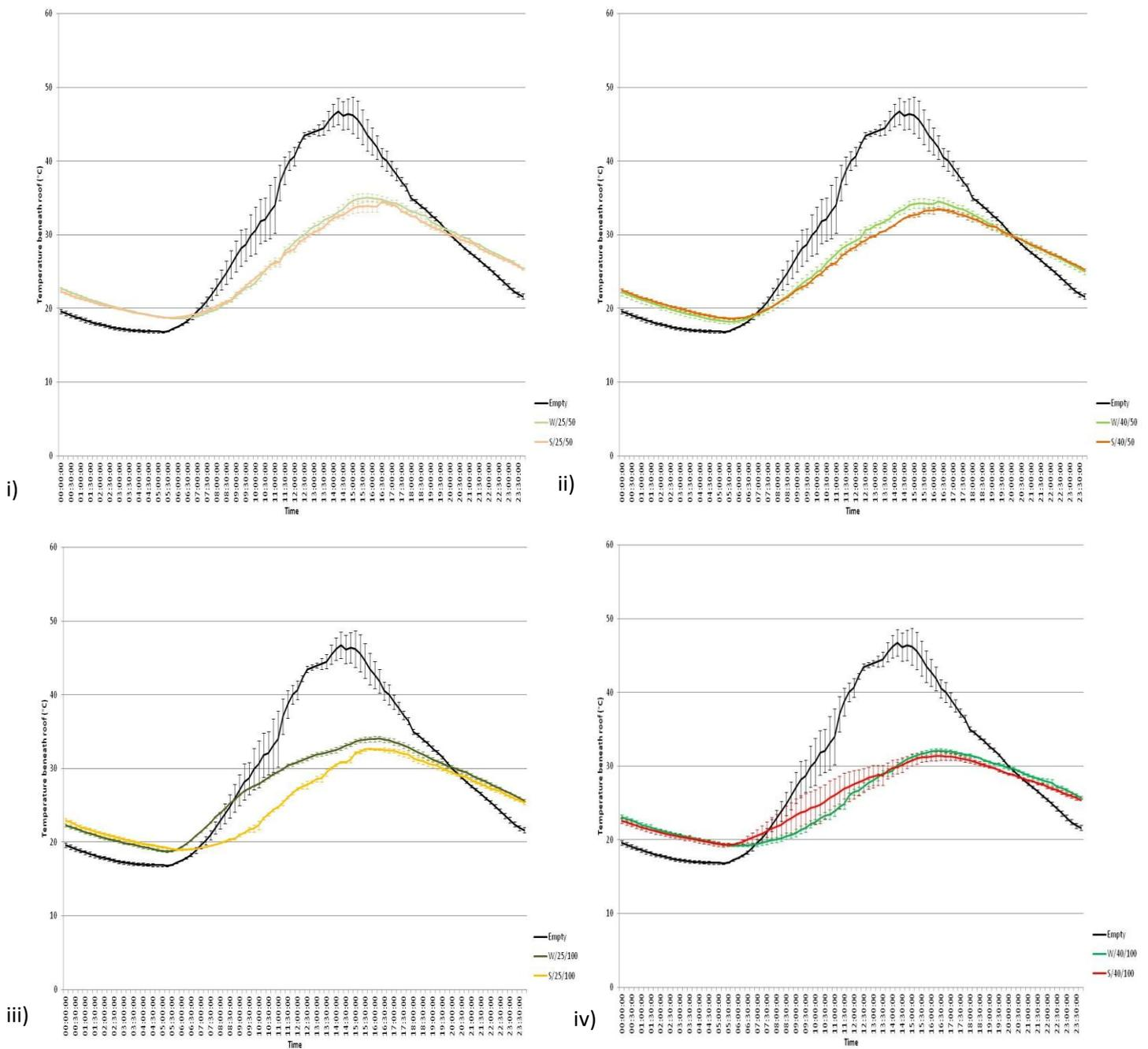
**Figure 22. Average temperature immediately beneath each green and control roofs at Barking Riverside on the hottest day of 2011 (27th June). i) Green roof pair W/25/50 and S/25/50; ii) Green roof pair W/40/50 and S/40/50; iii) Green roof pair W/25/100 and S/25/100; iv) Green roof pair W/40/100 and S/40/100. Error bars represent the standard error of the mean ( $n = 3$ ).**
