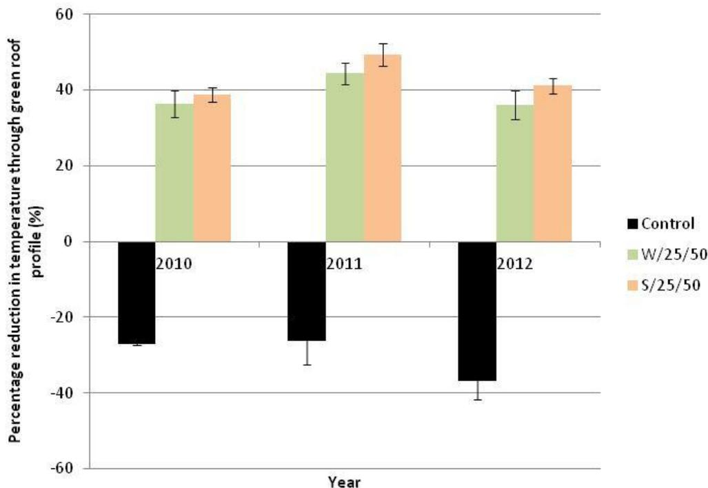
**Figure 25. Average percentage reduction in temperature through control, W/25/50 and S/25/50 green roof profiles for the month of July, 2010 to 2012.** Reduction in temperature calculated from the difference in temperature between sensor 4 (above the roof) and sensor 1 (beneath the roof). Error bars represent the standard error of the mean ( $n = 3$ ).
