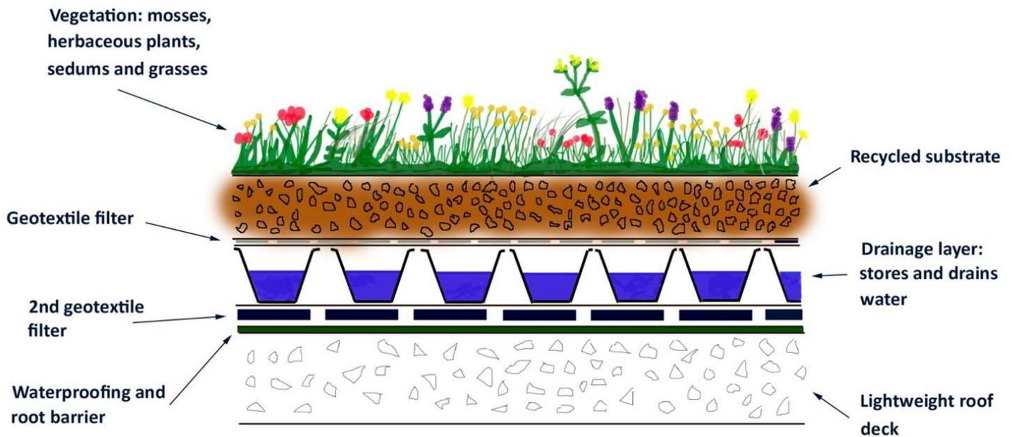
**Figure 1. Typical extensive green roof design**
