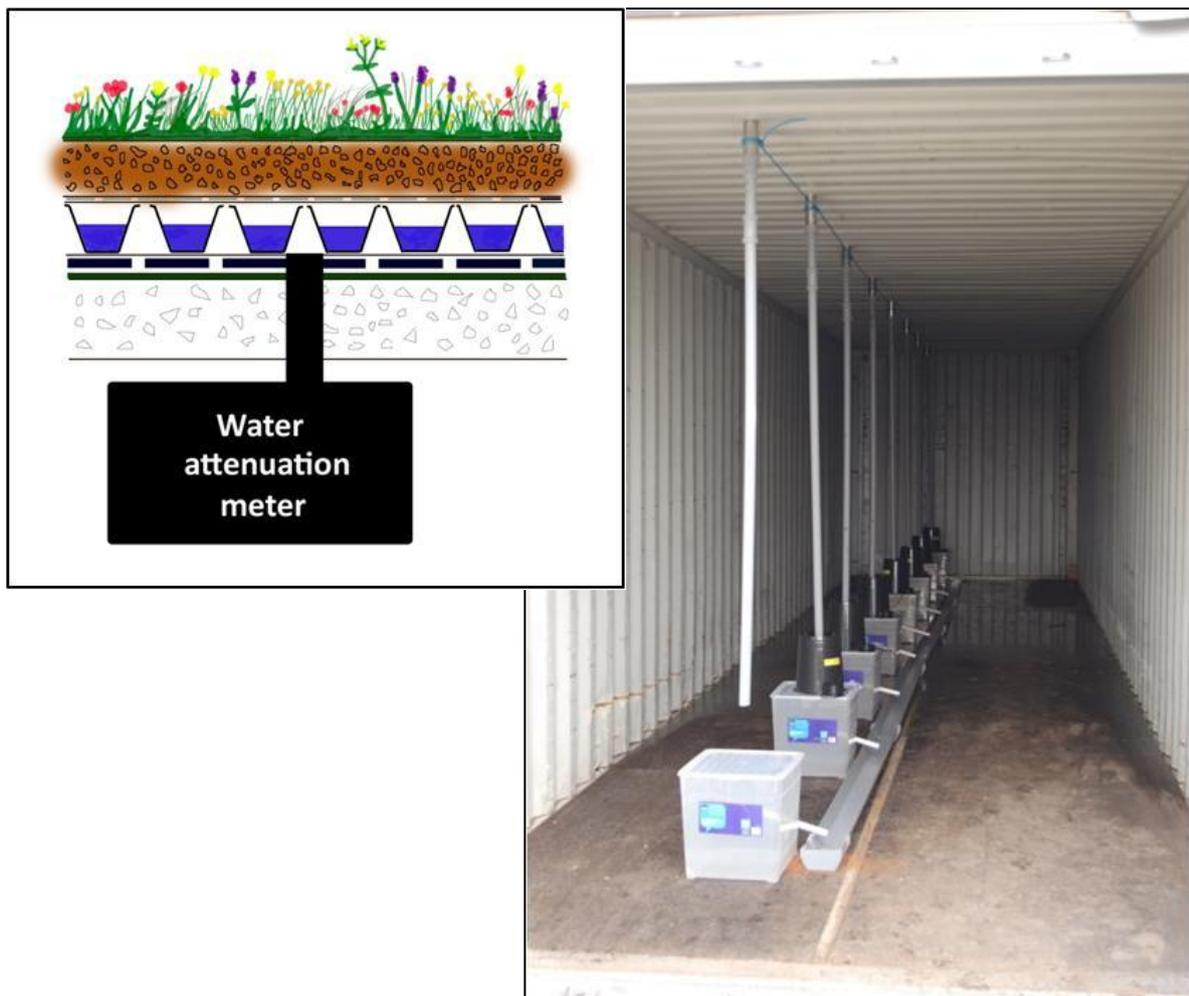
**Figure 6. Plan and image of rainfall runoff monitoring equipment beneath the green roof test bays at Barking Riverside Offices.**
