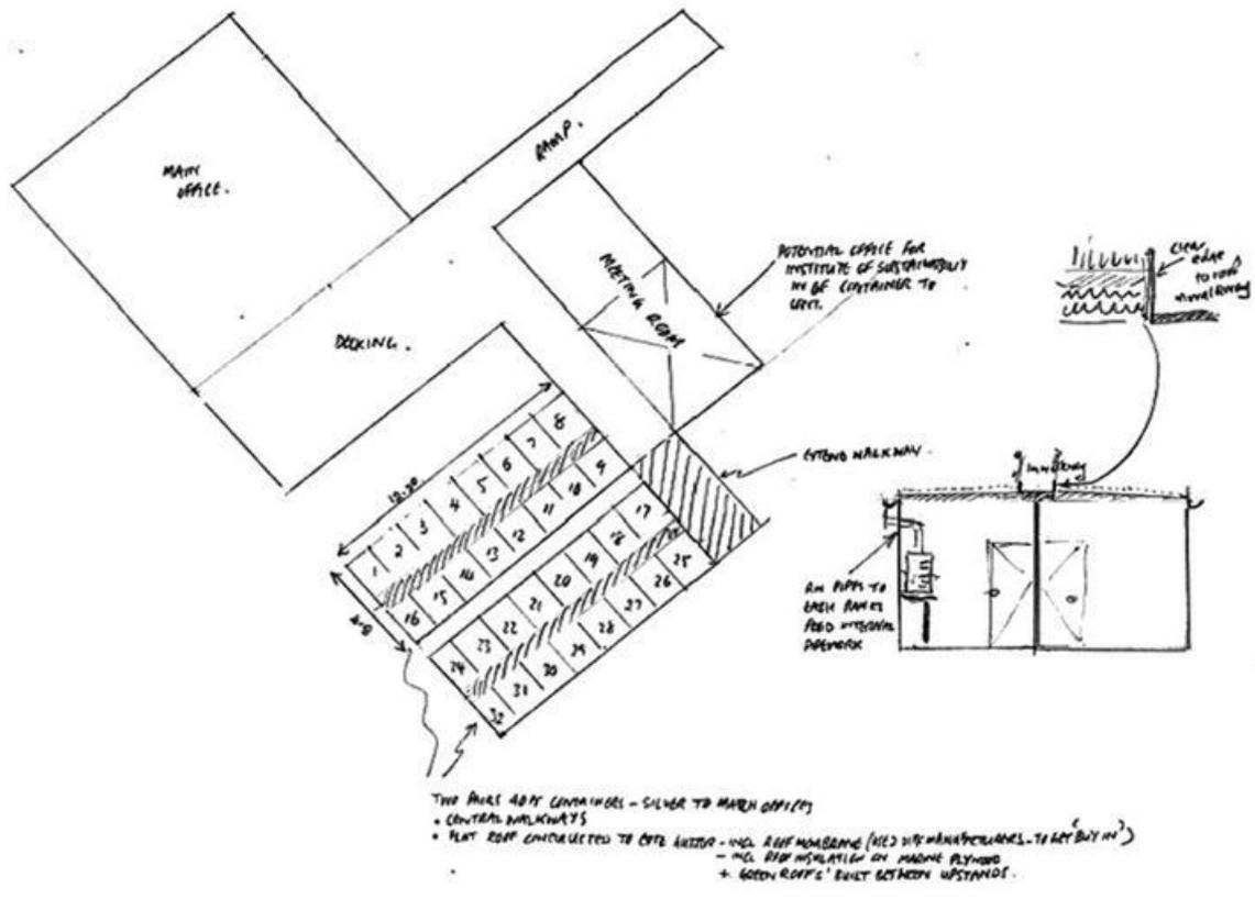
Figure 2. Plan of green roof test bays at Barking Riverside Offices.
