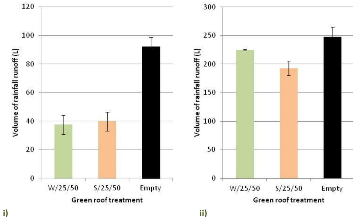
**Figure 13. Average percentage rainfall attenuation for empty control roofs and 25 mm drainage, 50 mm substrate sedum and wildflower roofs at Barking Riverside for i) the summer months July to September 2010, and ii) the winter months October to December 2010. Error bars represent the standard error of the mean ( $n = 3$ ).**
