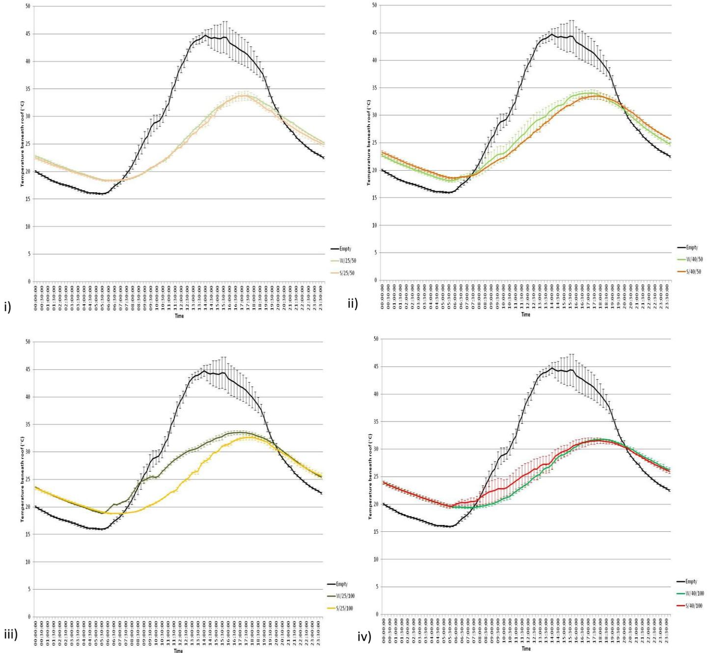
**Figure 21. Average temperature immediately beneath each green and control roofs at Barking Riverside on the hottest day of 2010 (9th July). i) Green roof pair W/25/50 and S/25/50; ii) Green roof pair W/40/50 and S/40/50; iii) Green roof pair W/25/100 and S/25/100; iv) Green roof pair W/40/100 and S/40/100. Error bars represent the standard error of the mean ( $n = 3$ ).**
