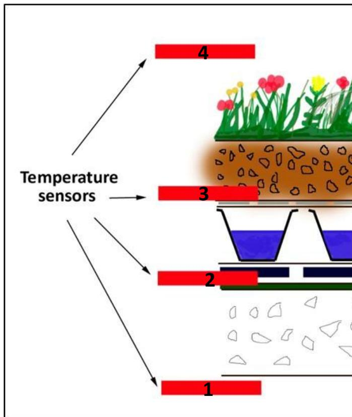
**Figure 7. Plan of temperature sensor monitoring equipment within the green roof test bay profiles at Barking Riverside Offices.**
