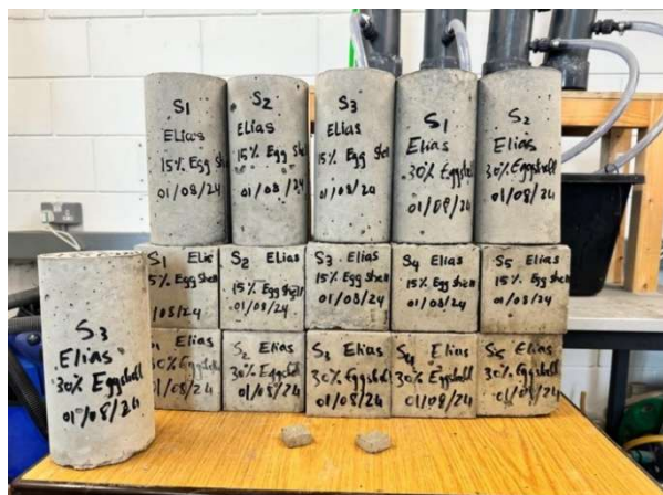
Fig. 2. Specimens with 15 % and 30 % eggshell powder immediately after unmoulding them.
