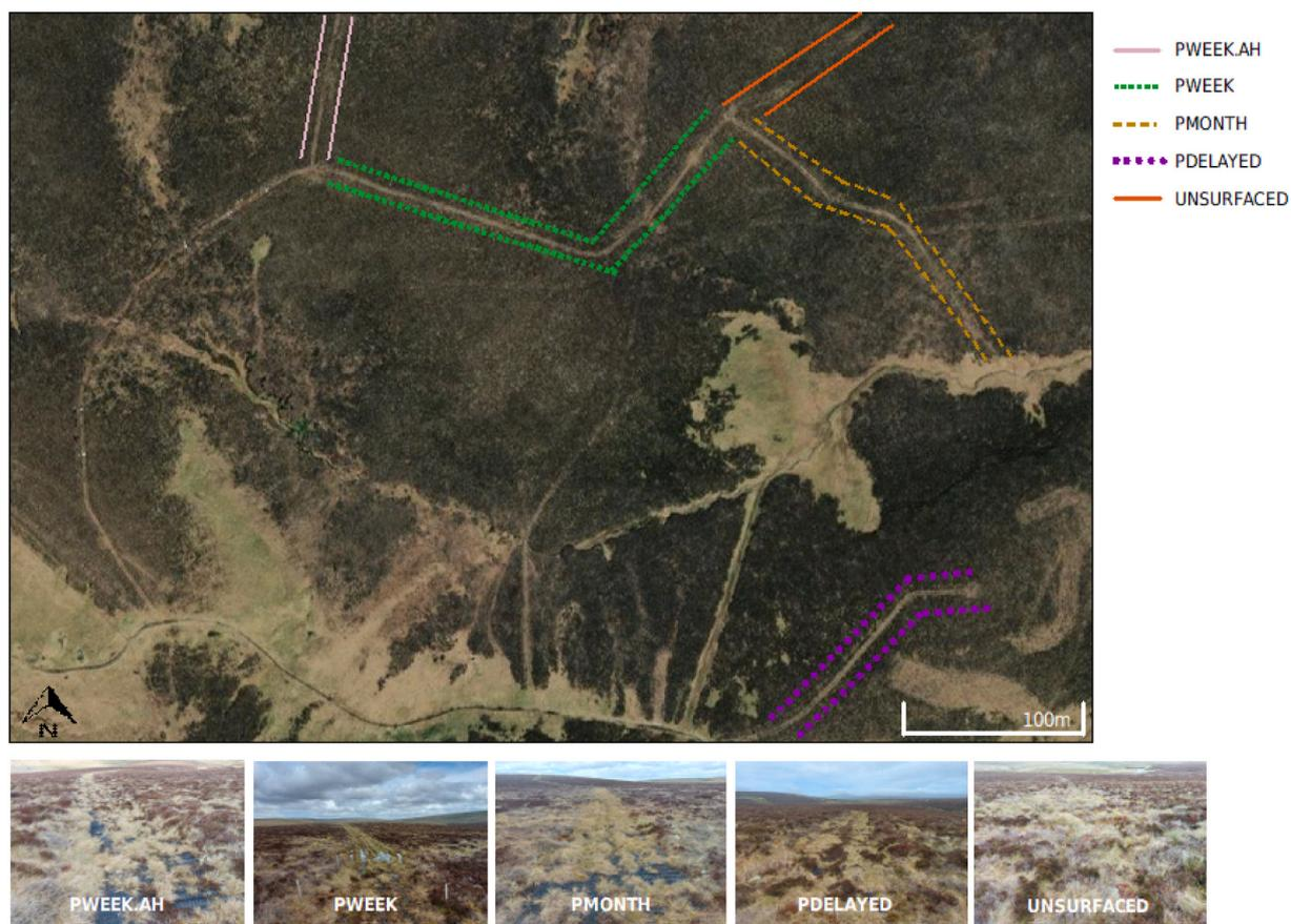
**Fig. 1.** Locations of the treatments on an aerial image from 2022 of the track sections (centre of image is at: 54.69298°N, 2.370061°W). Ground photographs of example sections of treatments are also shown, the track route can be seen in the centre of the paired lines, these are not indicative of the track width. The mean gradient of the tracks is 7.5%, although for PDELAYED the mean gradient is 5.0%.
