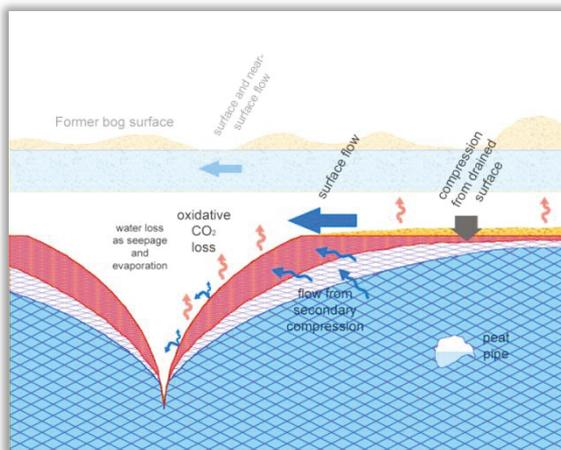
Prior to drainage, water typically occupied as much as 50% of the catotelm peat volume and loss of this water therefore **results in collapse and shrinkage of the peat adjacent to the drain. This process is called primary consolidation.** Its effects are felt immediately but may continue for some years. The key impact of this primary consolidation is that the drain, in effect, becomes wider because the ground immediately adjacent to the drain subsides.
