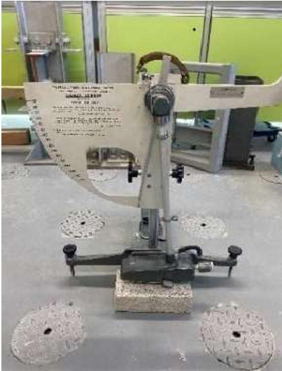
**Fig. 8.** Skid resistance test.
