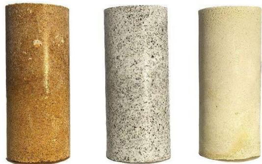
**Fig. 1.** Bioconcrete samples.
