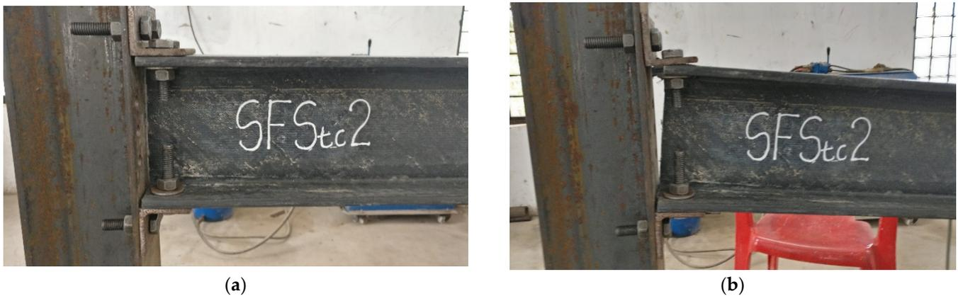
**Figure 14.** Shear-out failure in specimen SFStc2: (a) Undeformed joint; (b) Deformed joint.
