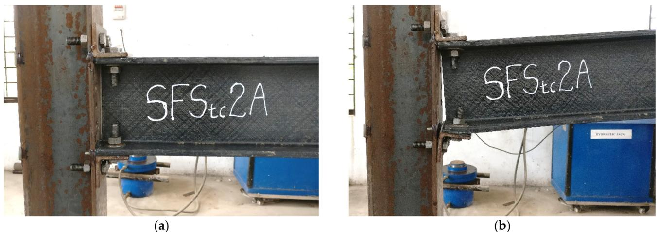
**Figure 15.** Adhesive debonding and shear-out failure in specimen SFStc2A: (a) Undeformed joint; (b) Deformed joint.
