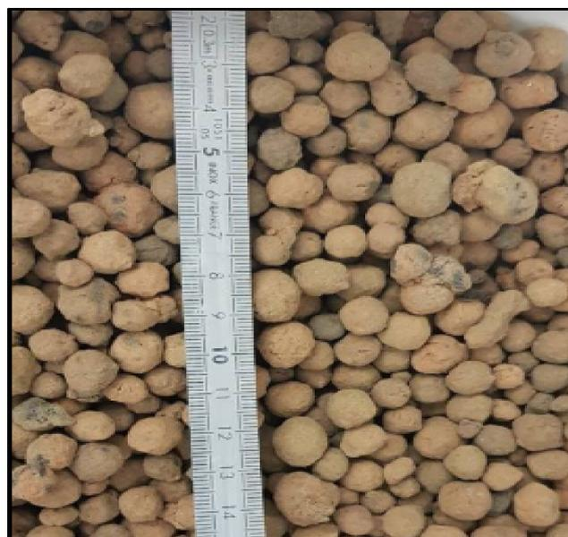
FIGURE 1 Coarse LYTAG aggregate.
