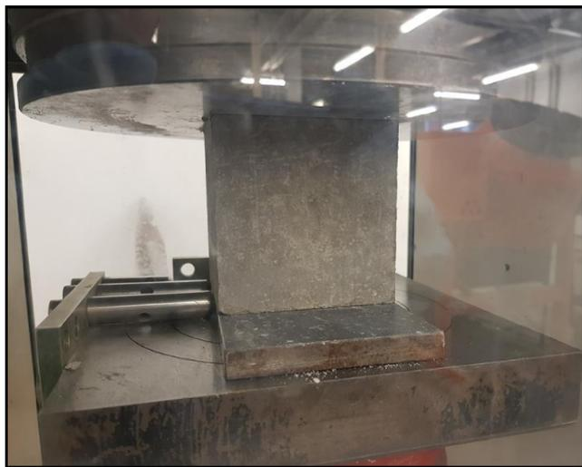
FIGURE 6 Crushing cube test.
