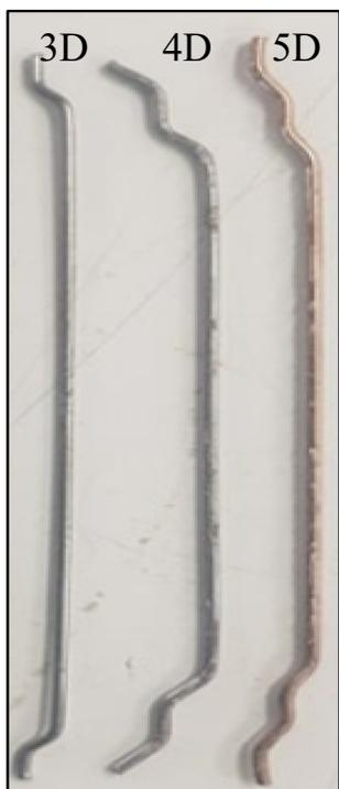
FIGURE 3 Fibers used in this work.
